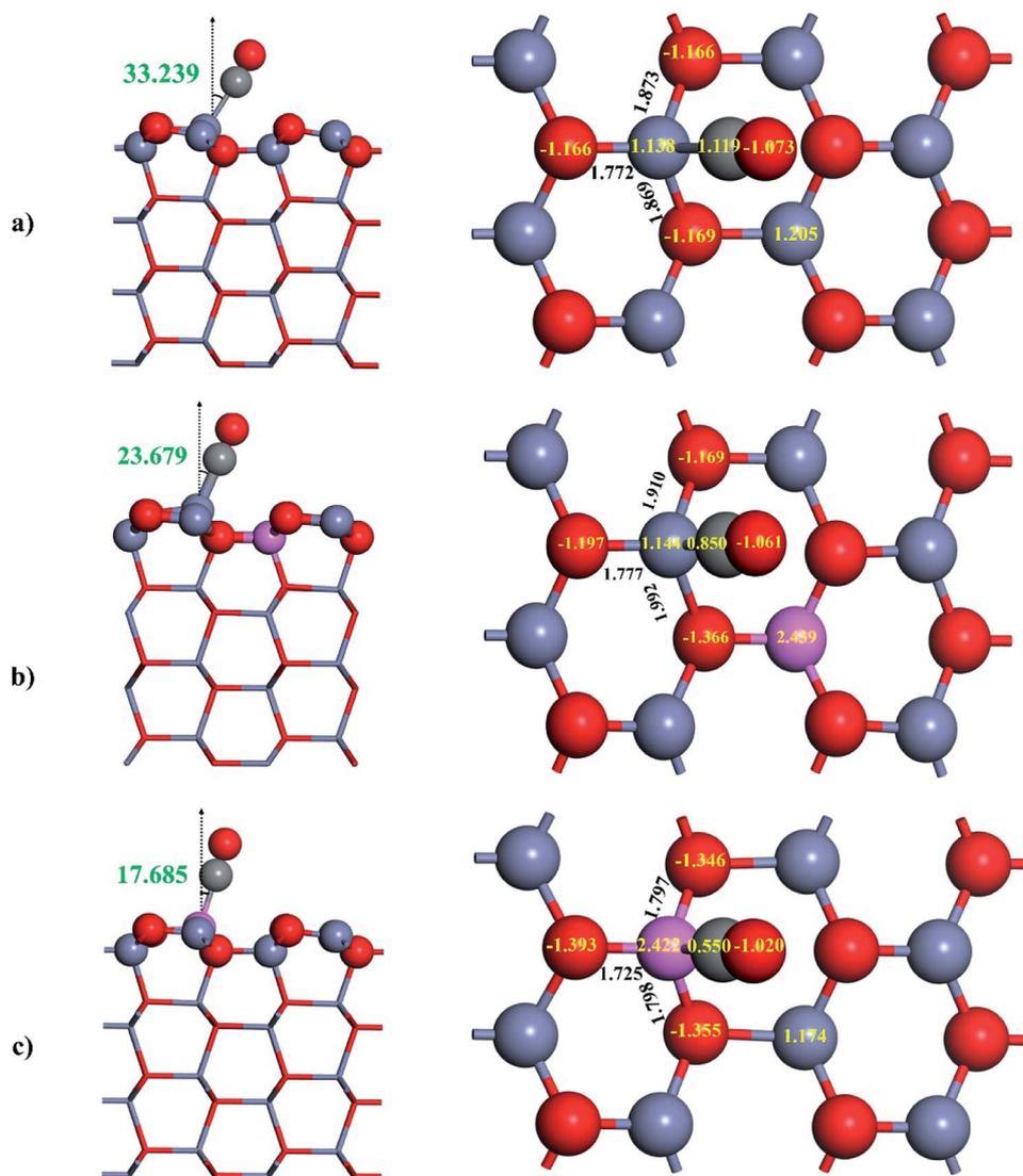
Fig. 3 Relaxed structure of adsorbed CO on: (a) ZnO(1010), (b) Al<sub>4c</sub>-doped ZnO(1010), (c) Al<sub>3c</sub>-doped ZnO(1010). The insert numbers in black, green and yellow colors are the values for the selected bond length, the bond angle and the effective Bader charge respectively.
