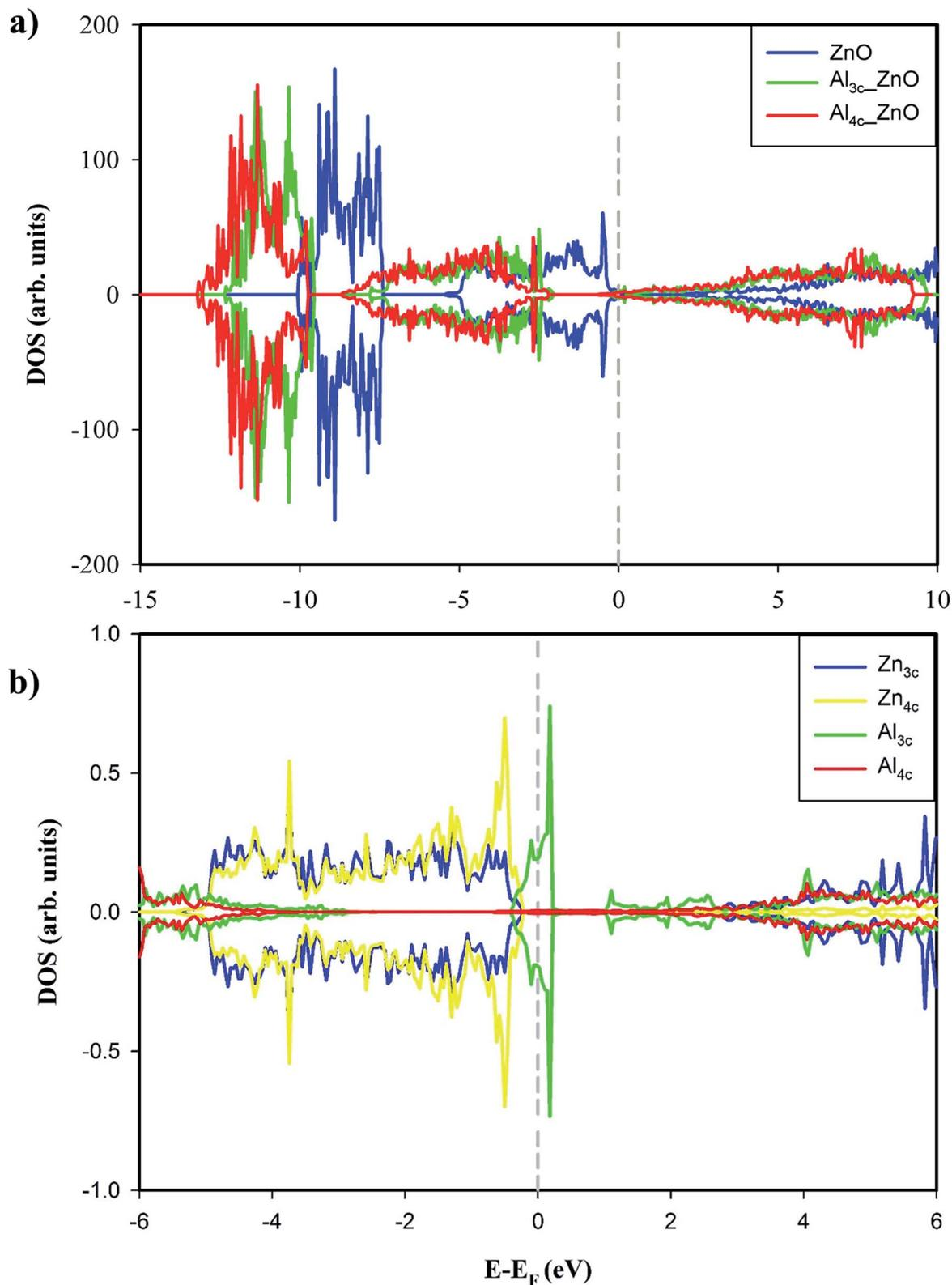
Fig. 2 (a) Total DOS of ZnO(1010),  $\text{Al}_{4c}$ -doped ZnO(1010) and  $\text{Al}_{3c}$ -doped ZnO(1010). (b) Projected DOS of  $\text{Zn}_{3c}$ ,  $\text{Zn}_{4c}$ ,  $\text{Al}_{3c}$  and  $\text{Al}_{4c}$ . The Fermi levels ( $E_F$ ) were shifted to 0 eV and indicated by the gray dashed lines.
