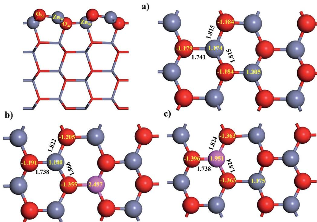
Fig. 1 Relaxed structure of: (a) ZnO(10 $\bar{1}$ 0), (b) Al<sub>3c</sub>-doped ZnO(10 $\bar{1}$ 0), (c) Al<sub>3c</sub>-doped ZnO(10 $\bar{1}$ 0). The insert numbers in black and yellow colors are the values for the bond length and the effective Bader charge.
