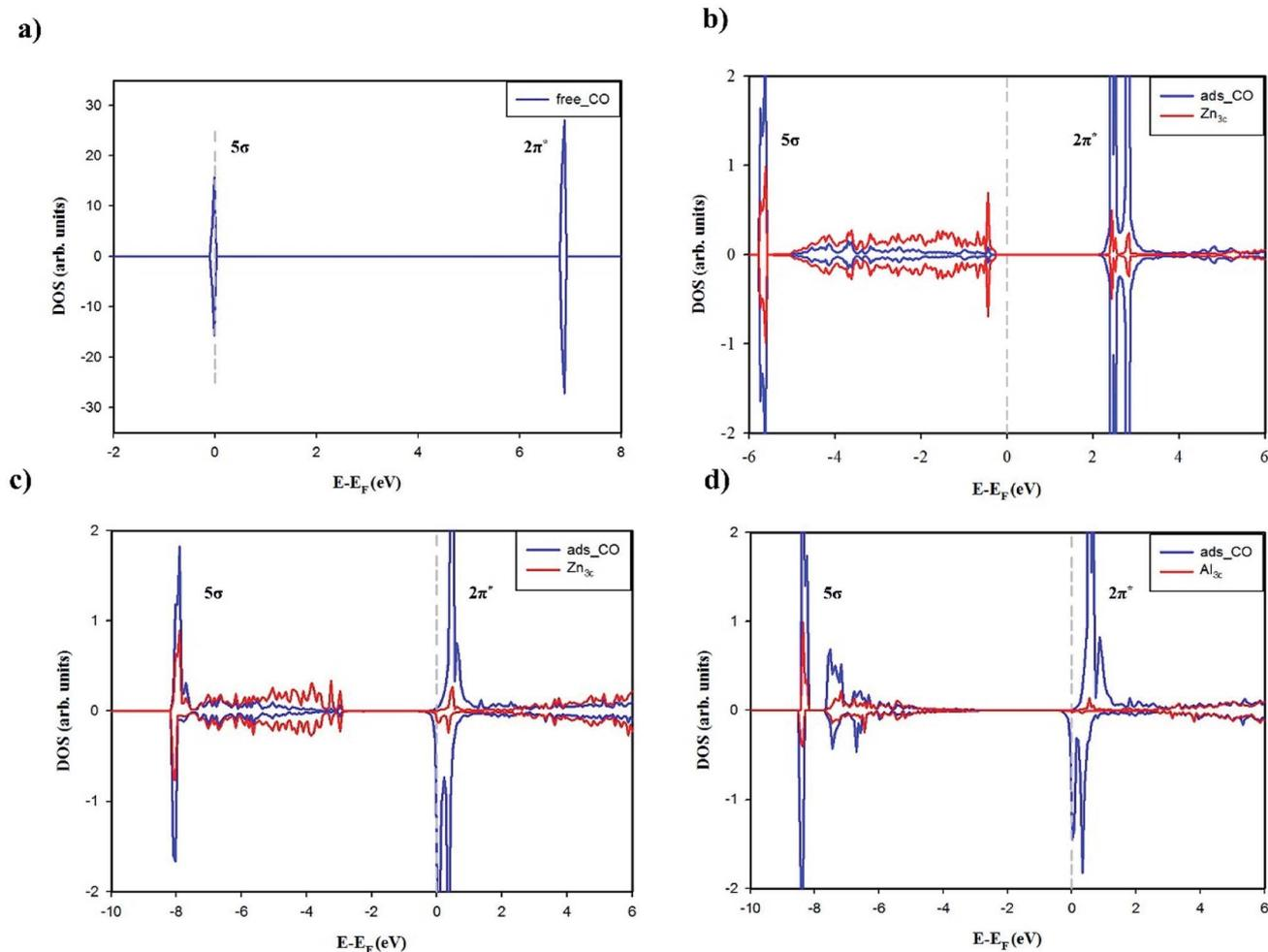
Fig. 5 Projected DOS for: (a) free CO, (b) adsorbed CO on ZnO(10 $\bar{1}0$ ), (c) adsorbed CO on Al<sub>4c</sub>-doped ZnO(10 $\bar{1}0$ ), (d) adsorbed CO on Al<sub>3c</sub>-doped ZnO(10 $\bar{1}0$ ). The Fermi levels ( $E_F$ ) were shifted to 0 eV and indicated by the grey dashed lines.
