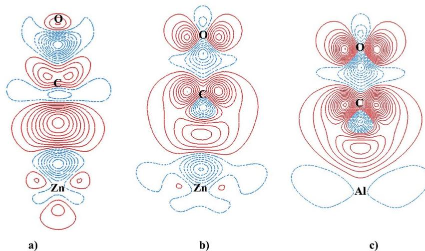
Fig. 6 Two-dimensional charge density difference contour plot for: (a) adsorbed CO on ZnO(10 $\bar{1}$ 0), (b) adsorbed CO on Al<sub>4c</sub>-doped ZnO(10 $\bar{1}$ 0), (c) adsorbed CO on Al<sub>3c</sub>-doped ZnO(10 $\bar{1}$ 0). The solid red line and dashed blue line represent an electron accumulation and an electron depletion respectively.
