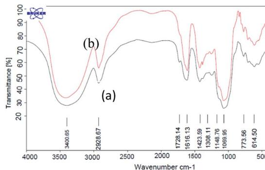
Fig. 1 FT-IR spectra of (a) GA (b) GA-OPO<sub>3</sub>H<sub>2</sub>.
