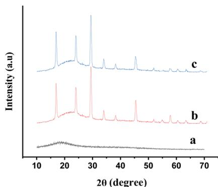
Fig. 3 XRD patterns of the (a) GA, (b) GA-OPO<sub>3</sub>H<sub>2</sub> and (c) reused GA-OPO<sub>3</sub>H<sub>2</sub>.
