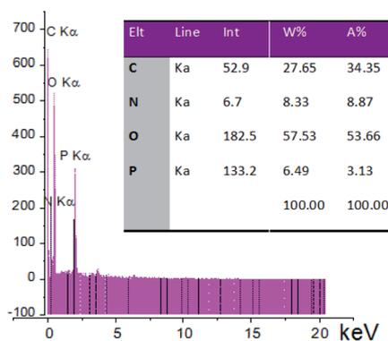
Fig. 4 EDS spectra of GA-OPO<sub>3</sub>H<sub>2</sub>.
