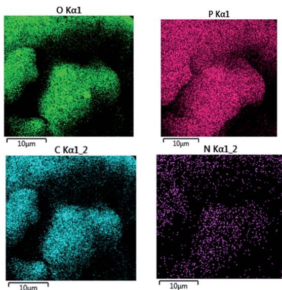
Fig. 5 Elemental mapping images of GA-OPO<sub>3</sub>H<sub>2</sub>.
