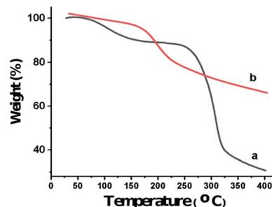
Fig. 6 Thermal gravimetric analysis pattern of (a) gum arabic, (b) GA-OPO<sub>3</sub>H<sub>2</sub>.
