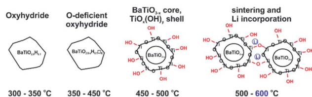
Fig. 6 Evolution of products from LiH reduction of \text{BaTiO}_3 with increasing synthesis temperature.
