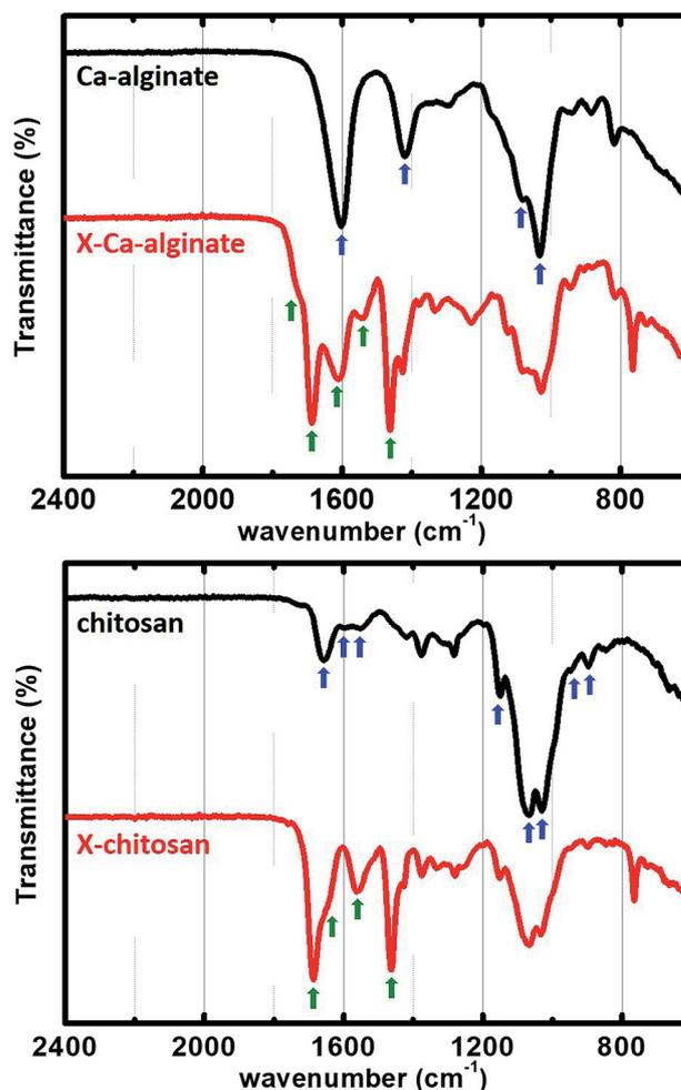
Fig. 5 ATR-FTIR spectra of native Ca-alginate and X-Ca-alginate aerogels (left), and native chitosan and X-chitosan aerogels (right).
