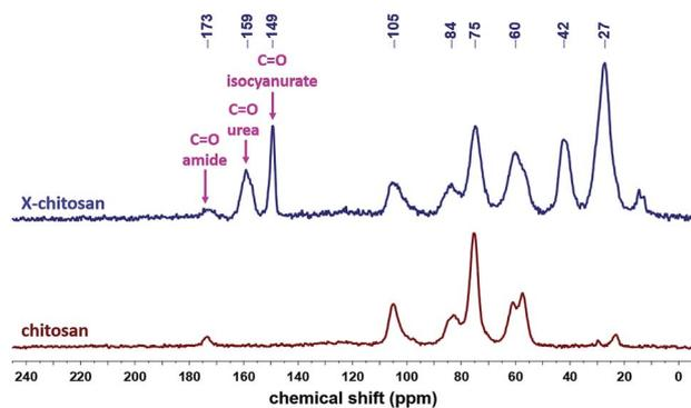
Fig. 7  $^{13}\text{C}$  CPMAS NMR spectra of native chitosan and X-chitosan aerogels, as indicated.
