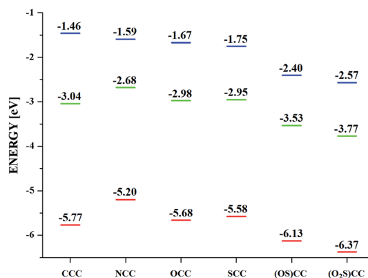
Fig. 10 Experimental energy diagram. HOMO level marked in red, LUMO in blue, and triplet state in green. HOMO and LUMO were derived from electrochemical oxidation and reduction, and the triplet state was estimated from the phosphorescence spectrum.
