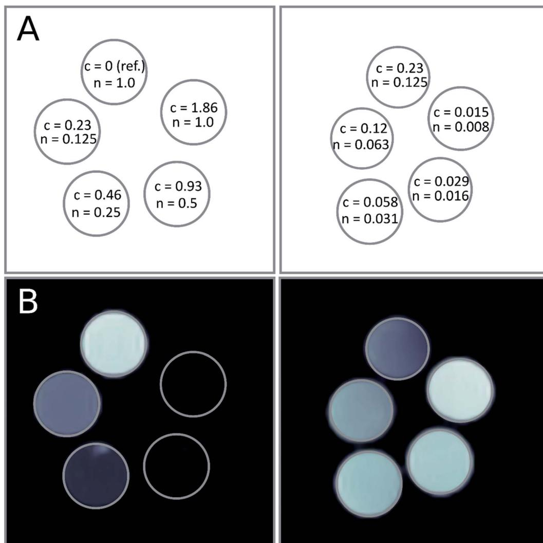
Fig. 5 (A) Arrangement of the samples in the scanner. (B) Axial images of samples containing different concentrations of SPIONs. RARE VTR sequence TE: 3.7 ms, TR: 5472 ms,  $n$  – number of nanocarriers [ $1.0 \times 10^{14} \text{ L}^{-1}$ ],  $c$  – SPIONs concentration [ $\text{mmol L}^{-1}$ ].
