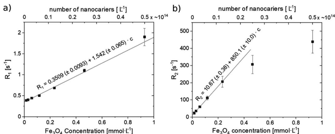
Fig. 7 Relaxation rate  $R_1$  (a) and  $R_2$  (b) of MN-PCL nanocarriers. Linear regression for  $R_1$  fit weighted with  $T_1$  uncertainties. Linear regression for  $R_2$  weighted with  $T_2$  uncertainties, in concentration range up to  $0.23 \text{ mmol L}^{-1}$ .
