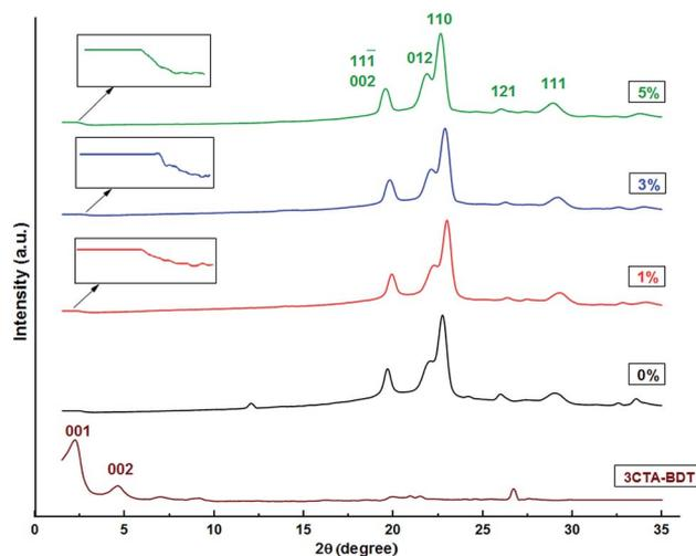
Fig. 1 XRD patterns for 3CTA-BDT, pure PBS and its nanocomposites PBS/ $y\%$  3CTA-BDT.
