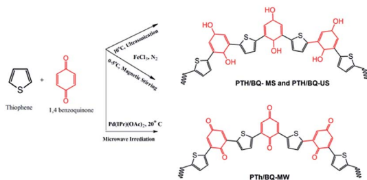
Scheme 1 Polymerization of PTh/BQ by different methods.
