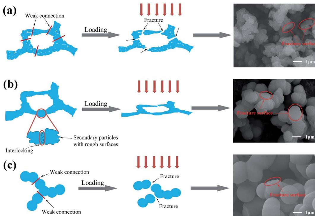
Fig. 5 Schematic of the structural change of the aerogel during compression: (a) D-0.27, (b) D-0.47 and (c) D-0.87.
