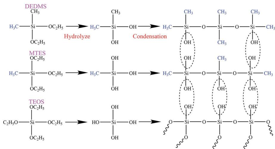
Fig. 1 Hydrolysis and condensation reactions of precursor.
