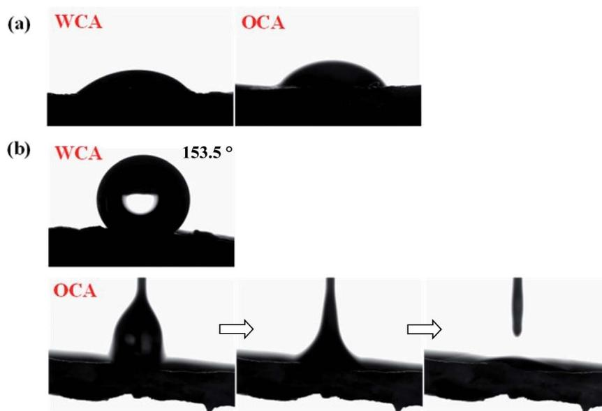
Fig. 5 The tests of contact angle for cellulose sponge before and after OTS modifying: (a) the images of water contact angle (WCA) and oil (chloroform) contact angle (OCA) on the control one, respectively, (b) the images of WCA and OCA on the modified one, respectively.
