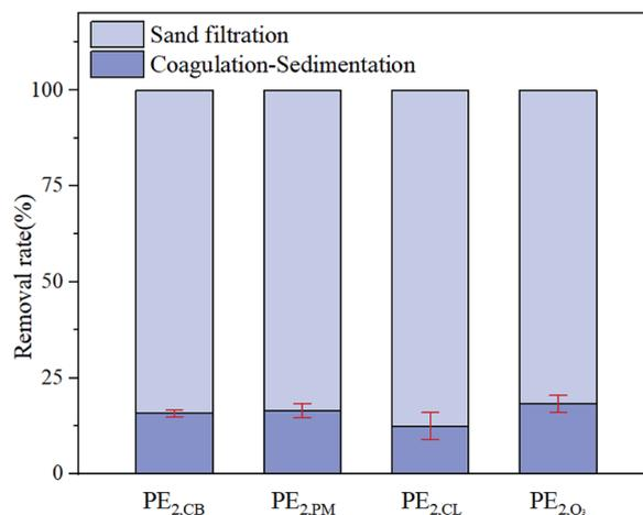
Fig. 5 Removal efficiency of PE MPs with conventional drinking water treatment processes. Experimental conditions: PE MP dosage 5 g L<sup>-1</sup>, PAC dosage 30 mg L<sup>-1</sup>, filtration rate 9 m h<sup>-1</sup> (EBCT = 5 min), pH = 7.0, 25 °C.
