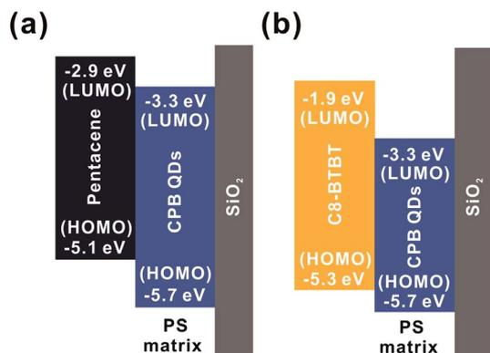
Fig. 5 The corresponding energy band diagrams of (a) CPB QDs/pentacene and (b) CPB QDs/C8-BTBT.
