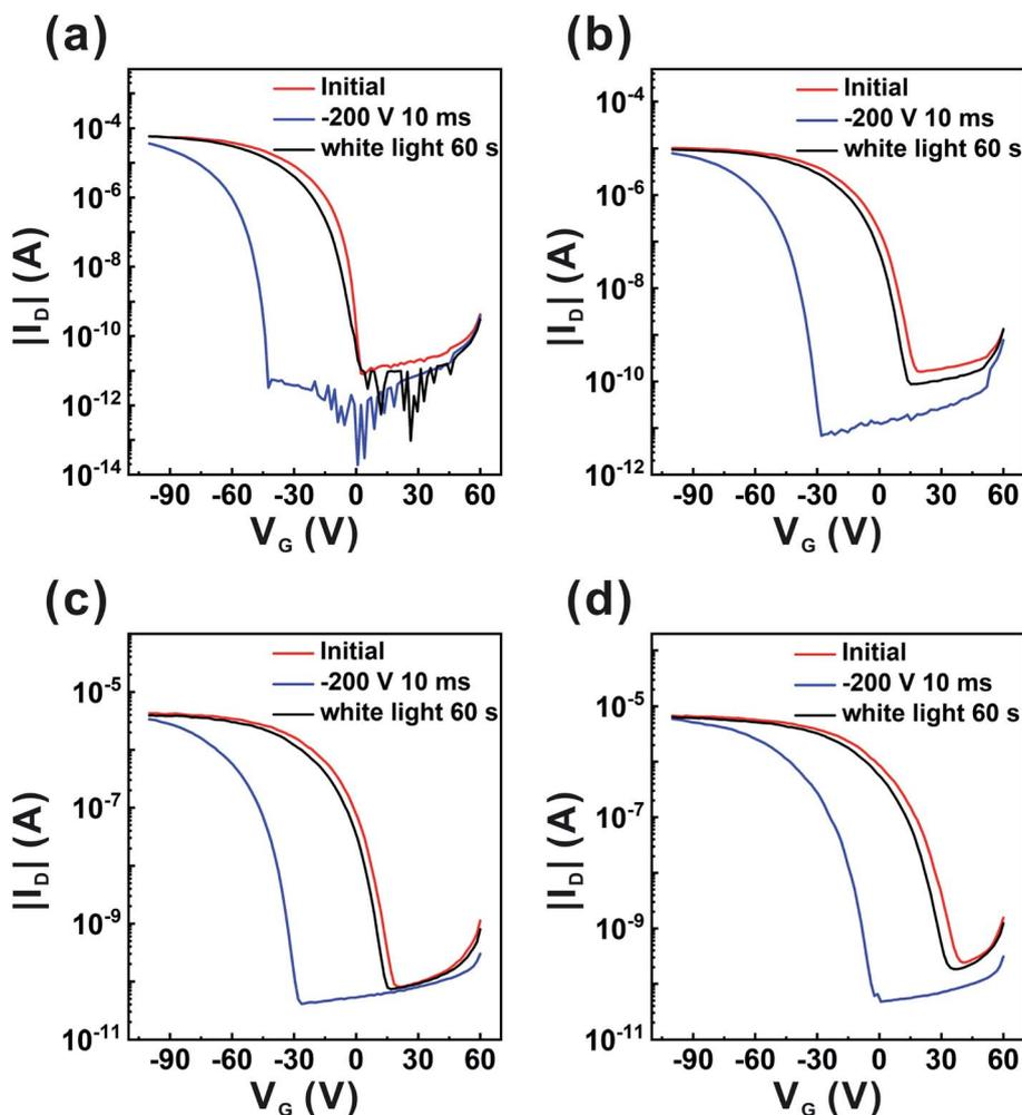
Fig. 2 Transfer characteristics ( $V_D = -40$  V) of the FGOFETs based on pentacene with CPB QDs/PS composite floating-gate layers. (a) CPB QDs/PS = 1 : 1, (b) CPB QDs/PS = 3 : 1, (c) CPB QDs/PS = 4 : 1, (d) CPB QDs/PS = 6 : 1.
