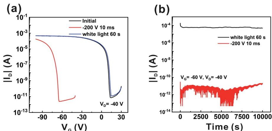
Fig. 3 (a) The transfer characteristics and (b) the retention characteristics of the FGOETMs based on C8-BTBT in electrical programming and photoinduced-reset states.
