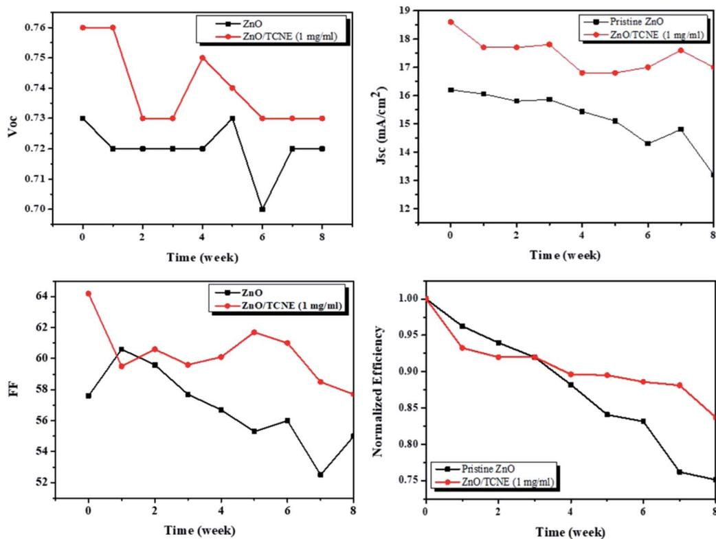
Fig. 10 (a) Normalized power conversion efficiencies of ZnO and ZnO/TCNE ETLs, respectively, devices as a function of eight weeks of storage time (b)  $I-V$  parameter breakdown of  $V_{oc}$ ,  $J_{sc}$ , FF, and PCE vs. time in eight weeks.
