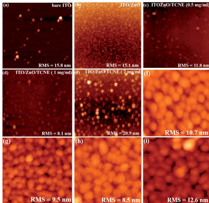
Fig. 6 Atomic force microscopy (AFM) ( $10 \times 10 \mu\text{m}^2$ ) surface images (a–e) showing RMS of bare ITO, pristine ZnO, and ZnO/TCNE (as 0.5 mg ml<sup>-1</sup>, 1 mg ml<sup>-1</sup>, and 2 mg ml<sup>-1</sup> of TCNE) films on ITO glass substrates and (f–i)  $5 \times 5 \mu\text{m}^2$  AFM images of PTB7:PC71BM blend films deposited on ZnO and ZnO/TCNE films.
