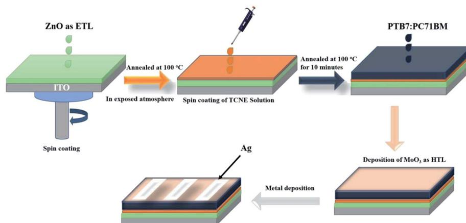
Fig. 1 Schematic representation of organic solar cell fabrication.
