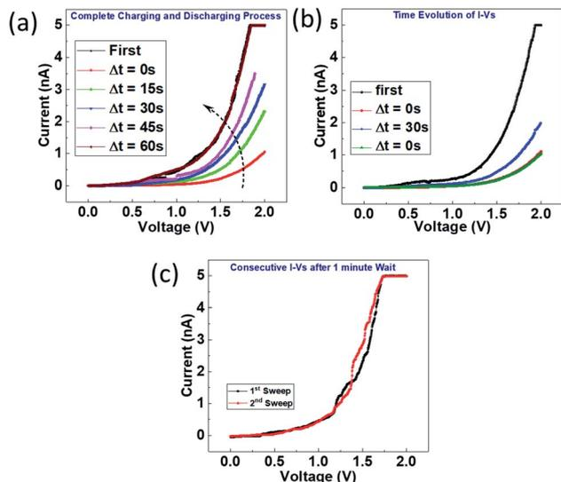
Fig. 6 The time-dependent  $I$ - $V$  measurements with (a) the complete charging and discharging process (b) the time-dependent voltage sweeps of 0 to +2 V (c) consecutive  $I$ - $V$ s with 1 minute time interval.
