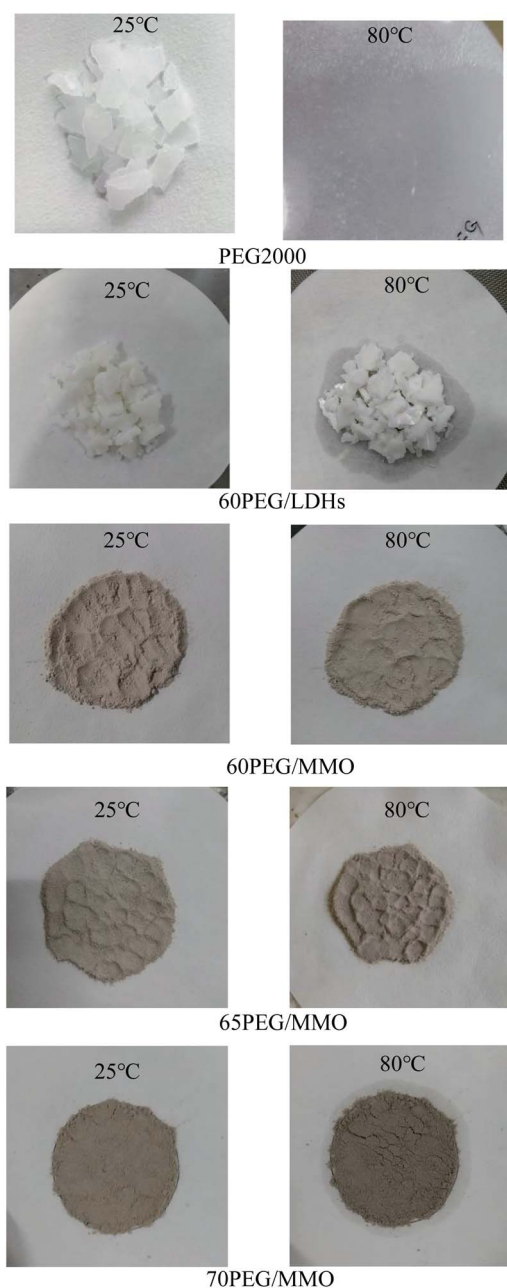
Fig. 1 Shape-stabilized property of a series of PEG-based PCMs at different temperatures.
