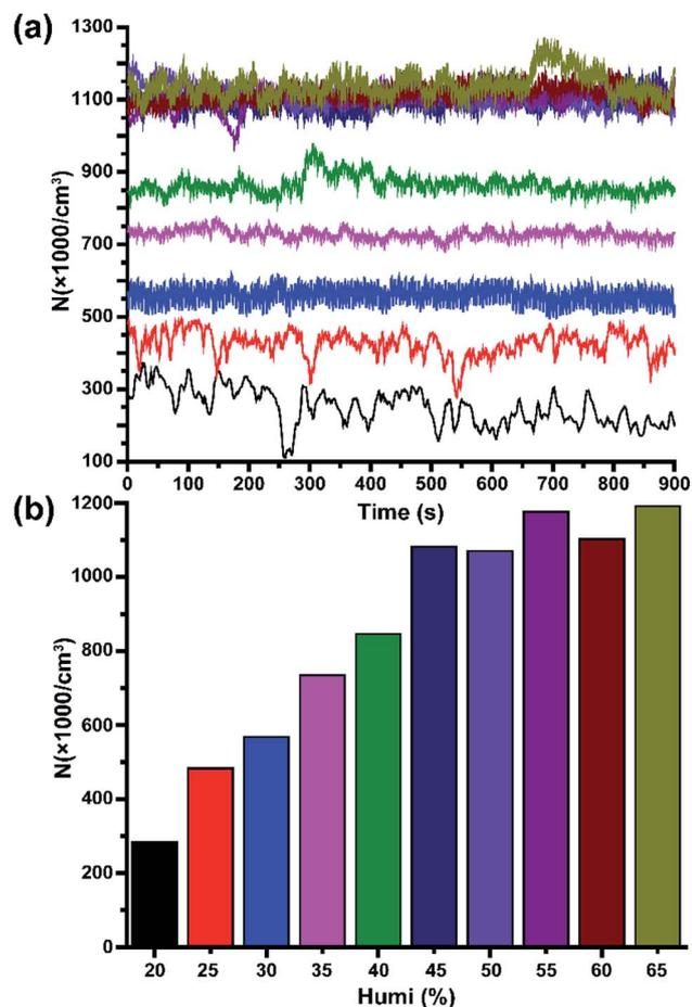
Fig. 4 Effect of relative humidity on the concentration and stability of HNAs. (a) Spectrum of HNAI concentration; (b) average HNAI intensity at different humidity.
