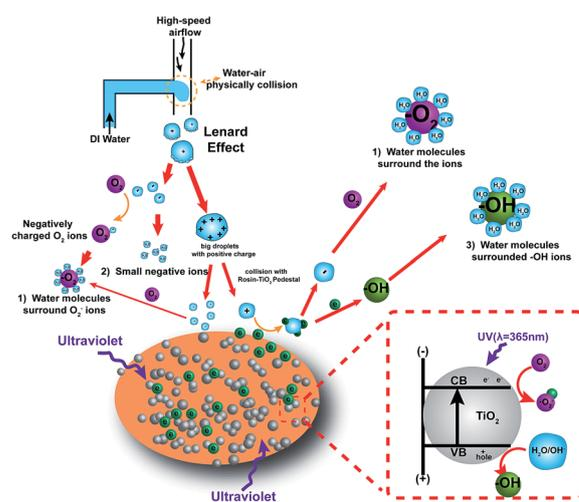
**Fig. 1** Schematic showing the rosin-TiO<sub>2</sub> photocatalytic materials for HNAI generation. The HNAIs including three parts: (1) water molecules surrounded O<sub>2</sub><sup>-</sup>, (2) small negative air ions, both (1) and (2) are come from Lenard effect; (3) water molecules surrounded OH<sup>-</sup>, part of (1) and (3) are generated by photoelectrons.
