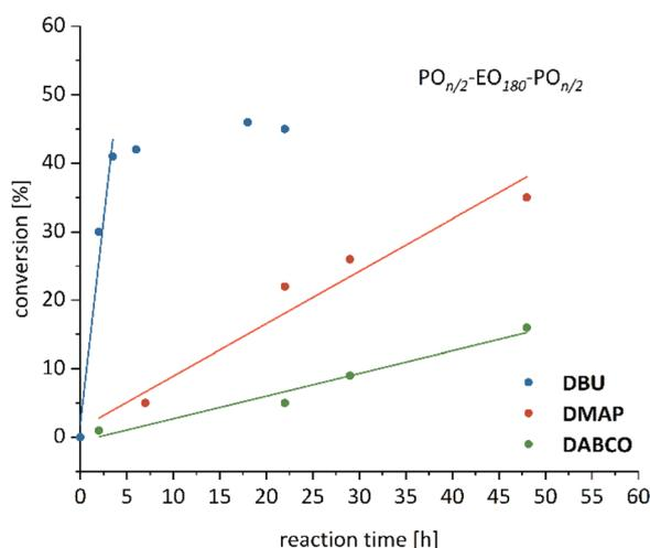
Fig. 4 Reaction time vs. conversion (<sup>1</sup>H NMR) for PO polymerization at 80 °C using organobase (5–7)/Et<sub>3</sub>B catalyst systems. Base/Et<sub>3</sub>B/PEO 8k [-OH]/PO = 1 : 4 : 5 : 1500 (molar ratio).
