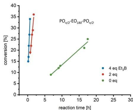
Fig. 2 Reaction time vs. conversion ( $^1\text{H NMR}$ ) for PO polymerization at  $80 \text{ }^\circ\text{C}$  using NHO **1** and different equivalents of  $\text{Et}_3\text{B}$  as cocatalyst:  $1/\text{PEO } 8\text{k } [-\text{OH}]/\text{PO} = 1 : 5 : 1500$ .
