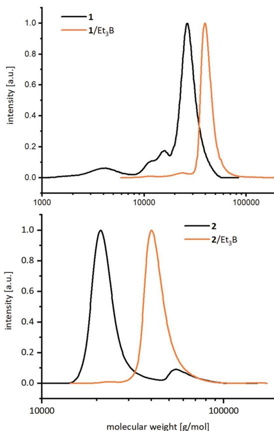
Fig. 3 Direct comparison of non-purified PO<sub>n/2</sub>-EO<sub>180</sub>-PO<sub>n/2</sub> derived from NHO alone (black) and NHO combined with 2.0 eq. of Et<sub>3</sub>B (orange). For reaction conditions, see Table 1, entries 1–4.
