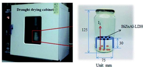
Fig. 1 Schematic of the device for the iodine adsorption experiments in static air.<sup>1</sup>
