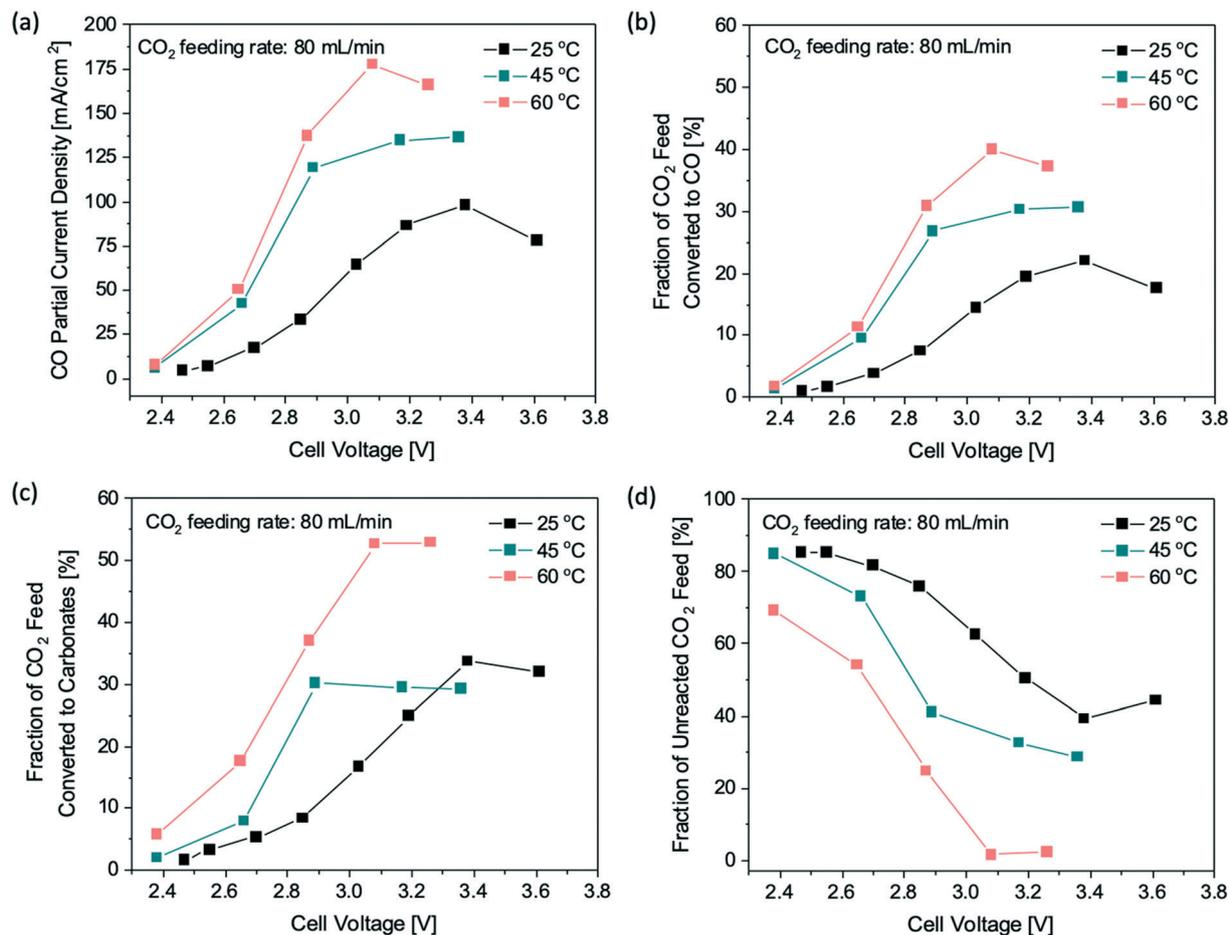
Fig. 3 Effects of reaction temperature on the CO<sub>2</sub> single-pass conversion at a fixed CO<sub>2</sub> feeding rate of 80 mL min<sup>-1</sup>: (a) CO partial current densities, (b) fraction of CO<sub>2</sub> feed being converted to CO via eCO<sub>2</sub>RR, (c) fraction of CO<sub>2</sub> feed consumed by the carbonate formation, and (d) fraction of unreacted CO<sub>2</sub> feed in the gas effluent at various cell voltages.
