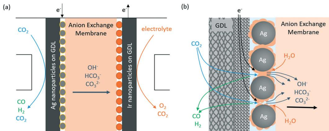
Fig. 1 Schematic diagrams of (a) the CO<sub>2</sub> flow electrolyzer configuration and (b) the cathode-membrane interface with multiple competing reactions.
