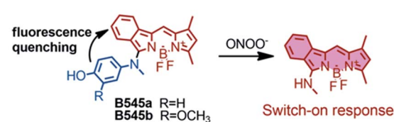
Fig. 1 Physicochemical-property guided fluorescent probe design for non-invasive imaging of \text{ONOO}^- during stroke in live mice. (a) Partition coefficients ( \log P ) of classical fluorophores were determined and benzo-BODIPY ( F4 ) was predicted to have a potentially good BBB permeability. (b) Electron-rich phenols may be oxidized to quinone by \text{ONOO}^- and this reaction has been used as a trigger for \text{ONOO}^- probe development. (c) Probes B545a and B545b were designed based on the F4 fluorophore which showed desirable \log P for BBB permeability. B545a and B545b were hypothesized to undergo a biocompatible reaction with \text{ONOO}^- to be transformed into highly fluorescent products.
