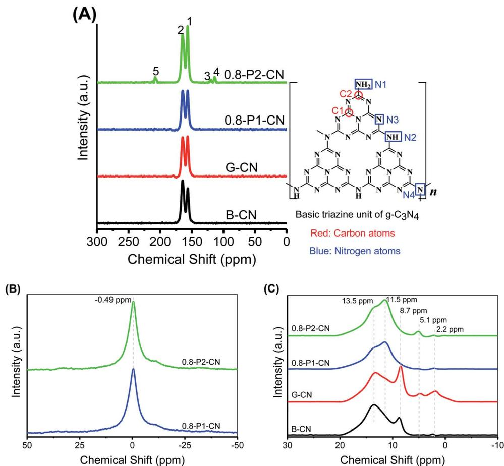
Fig. 3 (A) Solid-state NMR spectra of  $^{13}\text{C}$  and basic  $\text{g-C}_3\text{N}_4$  triazine unit structure. (B and C) Solid-state  $^{31}\text{P}$  and  $^1\text{H}$  NMR spectrums, respectively.
