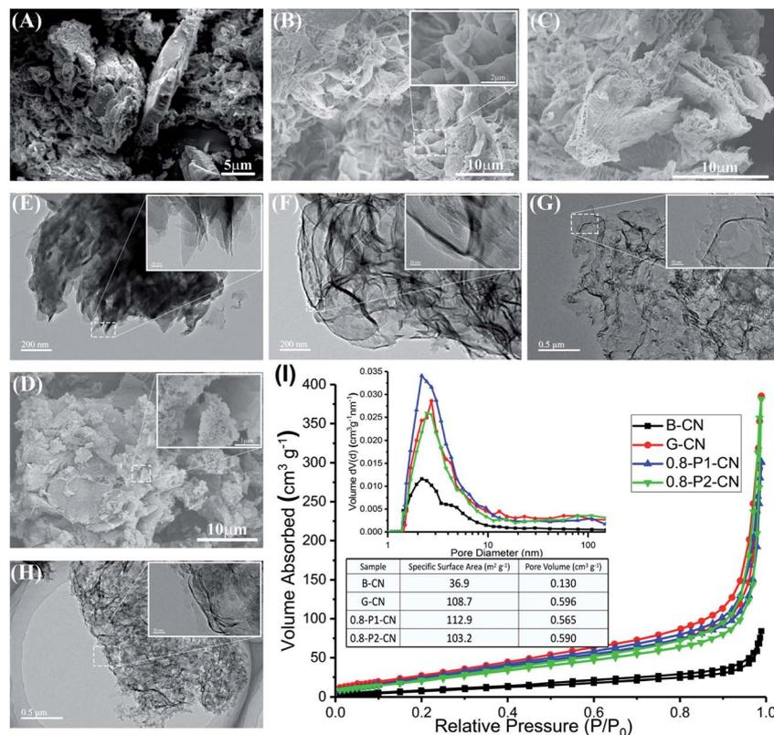
Fig. 1 (A, B, C and D) SEM images of B-CN, G-CN, 0.8-P1-CN and 0.8-P2-CN, respectively. (E, F, G and H) TEM images of B-CN, G-CN, 0.8-P1-CN and 0.8-P2-CN, respectively. (I) N<sub>2</sub> physisorption measurement results.
