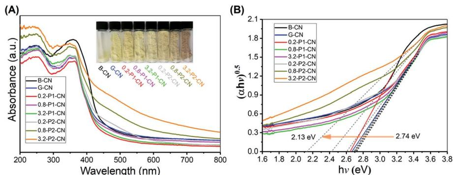
Fig. 7 (A) UV-Vis DRS spectra and. (B) Plots of transformed Kubelka–Munk function versus photon energy for a variety of g-C<sub>3</sub>N<sub>4</sub> samples.
