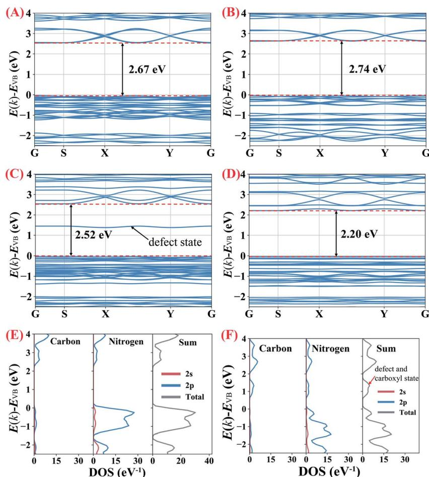
Fig. 8 (A–D) Calculated band structures of B-CN and g-C<sub>3</sub>N<sub>4</sub> with protonation, nitrogen vacancies and carboxyl groups, respectively. (E and F) corresponding PDOS for B-CN and g-C<sub>3</sub>N<sub>4</sub> containing nitrogen vacancies and carboxyl groups, respectively.
