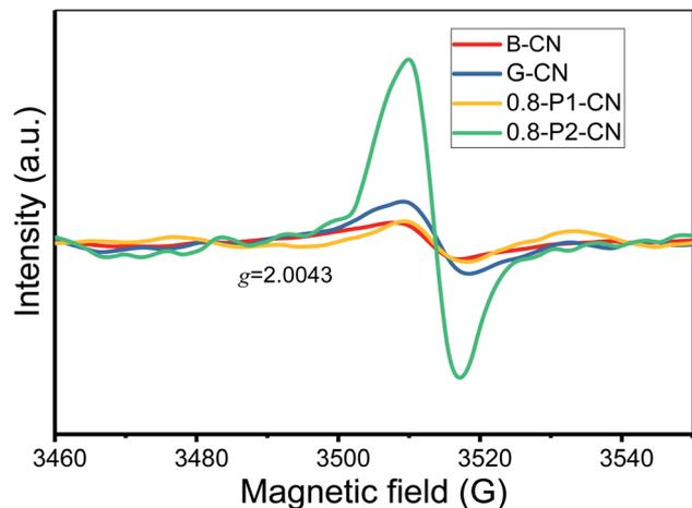
Fig. 5 EPR spectra of the representative  $g\text{-C}_3\text{N}_4$  samples.
