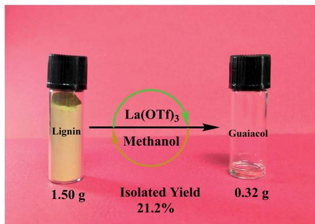
Fig. 4 Scale-up production of guaiacol from lignin. Reaction conditions: 1.50 g organosolv lignin, 0.6 g  $\text{La}(\text{OTf})_3$ , 120 mL methanol, 0.3 mL water, 270 °C, 0.1 MPa Ar, and 24 h.
