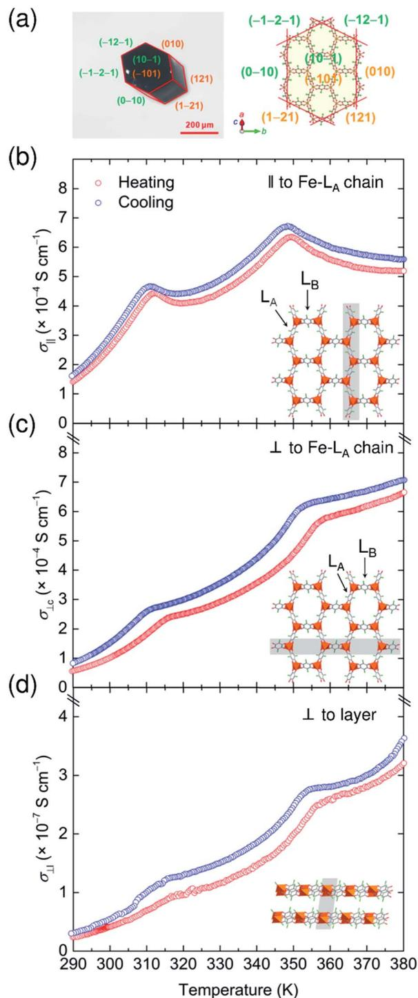
Fig. 8 Thermal variation of single-crystal electronic conductivity for **1-d** using a typical size of hexagonal crystals (a), in which gold wire probes were attached parallel ( $\parallel$ ; b) and perpendicular ( $\perp_c$ ; c) to the Fe–L<sub>A</sub> chains in the layer, and perpendicular to the layer-stacked direction ( $\perp_l$ ; d).
