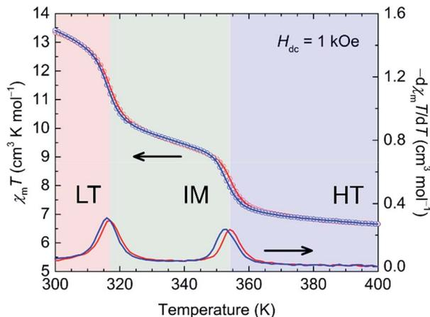
Fig. 4 Temperature dependence of  $\chi_m T$  and  $-d(\chi_m T)/dT$  for **1-d** measured at  $H_{dc} = 1$  kOe continuously between 300 K and 400 K in initial heating (red) and post-cooling (blue) processes, where the LT, IM, and HT phases are displayed as red, green, and blue areas, respectively.
