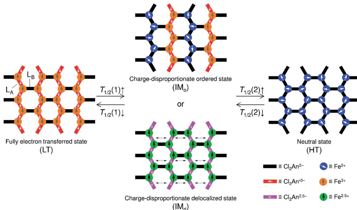
Scheme 1 Schematic illustrations of the variations of charge-ordered states in **1** and **1-d**, where the fully electron transferred state, charge-disproportionate ordered state, charge-disproportionate delocalized state, and neutral state are represented as LT,  $IM_o$ ,  $IM_d$ , and HT phases, respectively.
