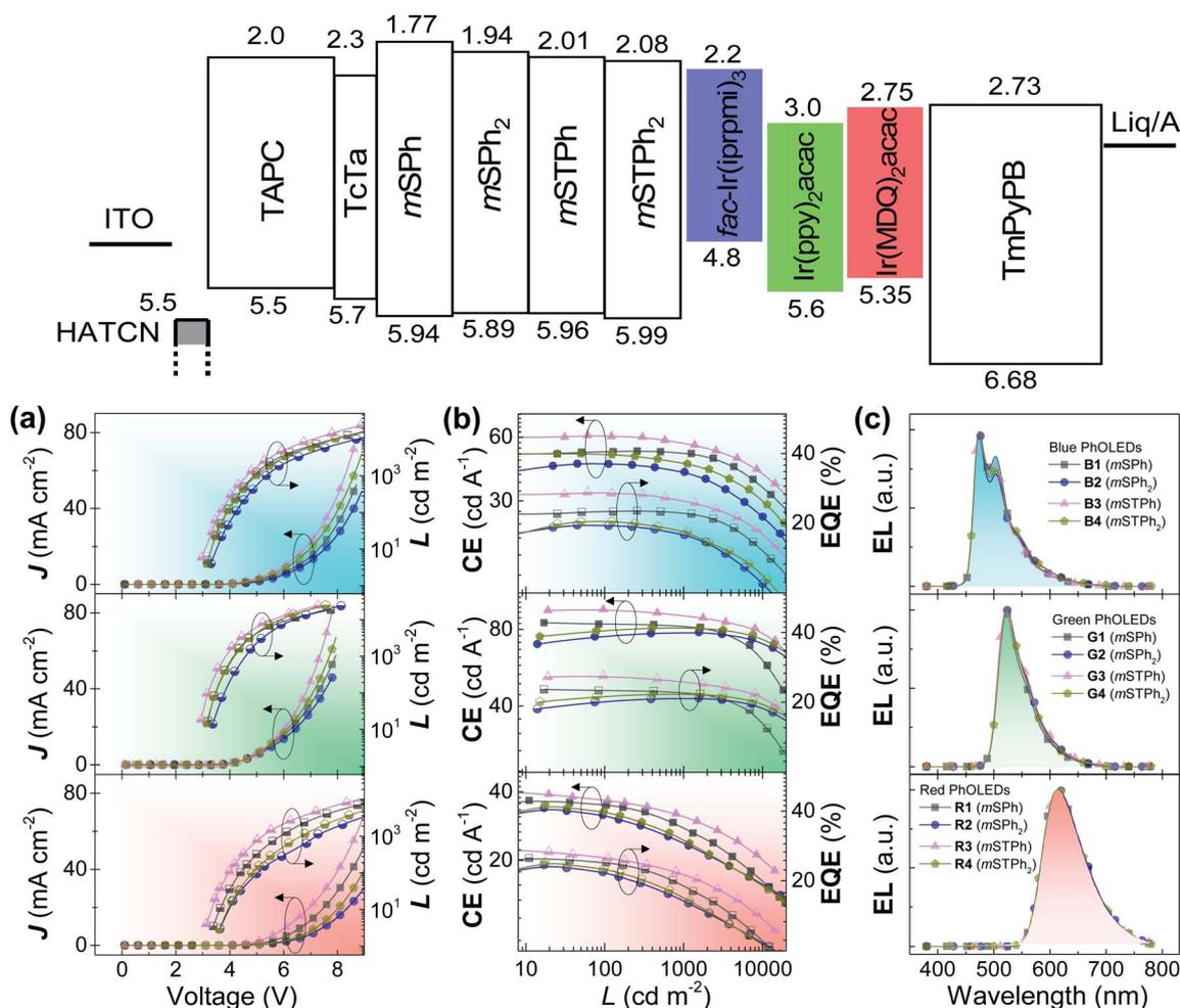
Fig. 4 The energy diagram and performance of the devices. (a) Current density–voltage–luminance ( $J$ – $V$ – $L$ ) curves, (b) current efficiency–luminance–external quantum–efficiency ( $CE$ – $L$ – $EQE$ ) curves, and (c) EL spectra of the blue (Top), green (Middle) and red (Bottom) PhOLEDs at a current density of 10  $mA cm^{-2}$ .
