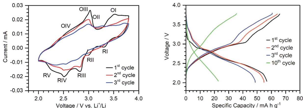
Fig. 4 Left: cyclic voltammograms of  $\{\text{Ca}_2\text{V}_{12}\}$ -based electrodes in the range of 2.0–3.8 V vs.  $\text{Li}^+/\text{Li}$  at a scan rate of 0.2  $\text{mV s}^{-1}$ . Right: voltage profile of  $\{\text{Ca}_2\text{V}_{12}\}$  half-cells cycled between 2.0 and 3.8 V vs.  $\text{Li}^+/\text{Li}$  with a constant current density of 50  $\text{mA g}^{-1}$  at 25 °C.
