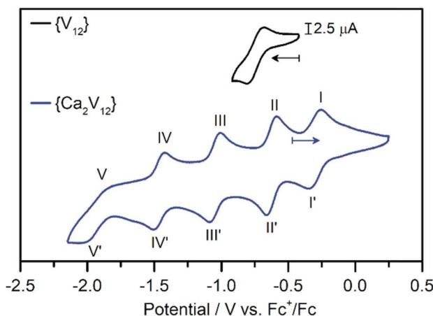
Fig. 2 Cyclic voltammograms of  $\{\text{Ca}_2\text{V}_{12}\}$  (blue) and  $\{\text{V}_{12}\}$  (black). Conditions: anhydrous, deoxygenated DMF containing 0.1 M  $(n\text{Bu}_4\text{N})\text{PF}_6$  as the supporting electrolyte (scan rate:  $0.1 \text{ V s}^{-1}$ ), [cluster]: 1 mM.
