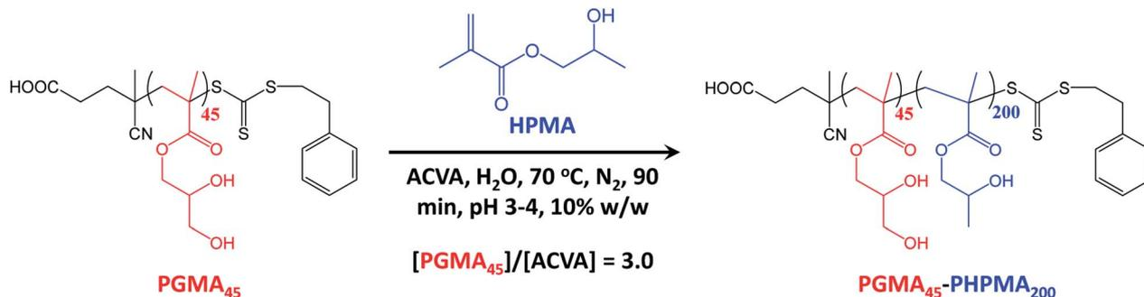
Fig. 2 Synthesis of  $\text{PGMA}_{45}\text{-PHPMA}_{200}$  diblock copolymer nano-objects via RAFT aqueous dispersion polymerization of HPMA using a water-soluble  $\text{PGMA}_{45}$  precursor block at 70 °C and targeting a PHPMA DP of 200.
