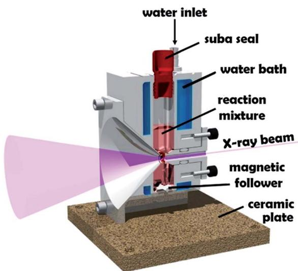
**Fig. 1** Schematic cross-section of the stirrable reaction cell used for *in situ* SAXS experiments performed during RAFT aqueous dispersion polymerization of HPMA at 70 °C. The volume of the reaction solution within this cell is approximately 2.0 mL, which is sufficient to enable *postmortem* analysis using multiple characterization techniques. Figure reprinted with permission.<sup>61</sup>
