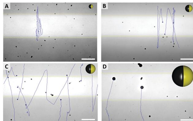
**Fig. 4** Typical pathways of particles, with different average sizes ((A) 0.7  $\mu\text{m}$ , (B) 1.2  $\mu\text{m}$ , (C) 1.6  $\mu\text{m}$ , (D) 3.5  $\mu\text{m}$ ) and particle sketches in relative sizes (see Videos in ESI,† S1–S4). Scale bar 25  $\mu\text{m}$ .
