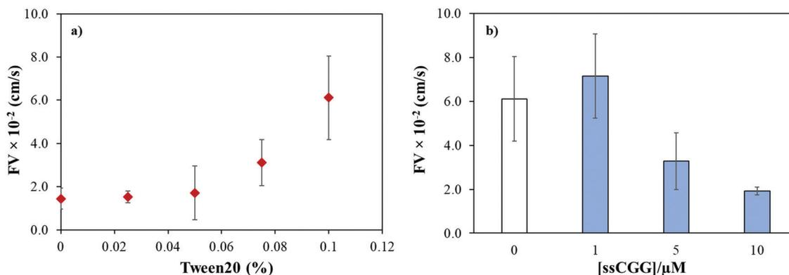
**Fig. 2** (a) Effect of surfactant concentration (Tween 20) on flow velocity of PBS buffer (pH 7.4) in wax-on-plastic microchannel. (b) Flow velocity of single-stranded CGG-8 at different concentrations prepared in PBS buffer containing 0.1% Tween 20. Error bar represent standard deviation for three replicates.
