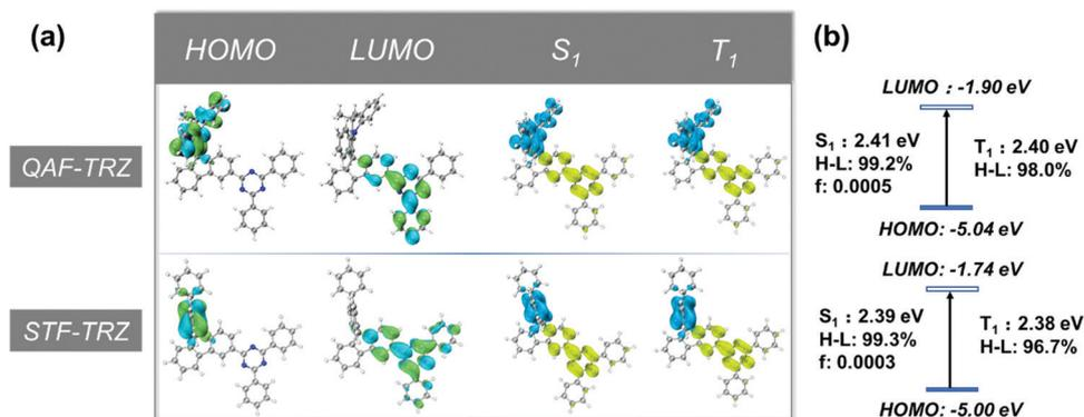
Fig. 1 (a) The distribution of HOMOs and LUMOs and the analysis for distribution of hole (blue), electron (yellow) for  $S_1$  and  $T_1$  and (b) energy level diagram of HOMOs, LUMOs,  $S_1$  and  $T_1$ .
