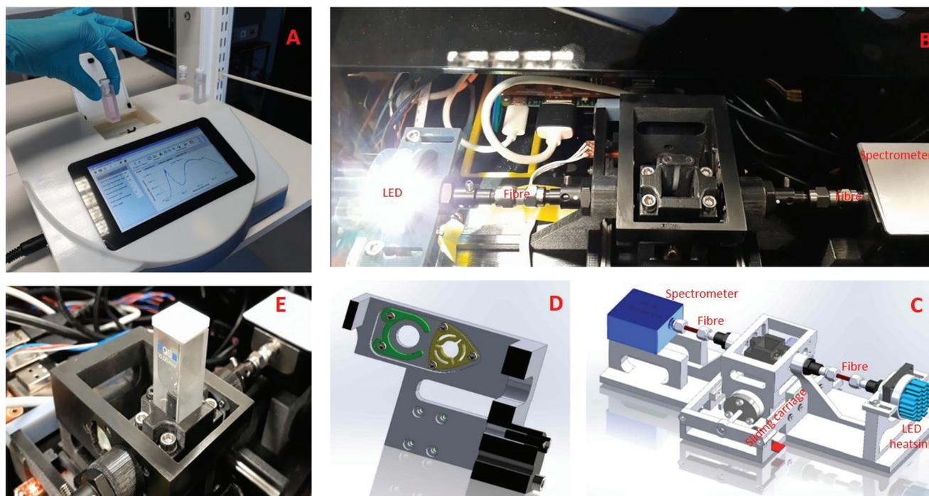
**Fig. 1** (a) CEA spectrometer with 1 cm cuvette to show scale with structural elements fabricated using i3DP (b and c) horizontal optical cavity showing the led, fibre coupling, sample holder and sliding carriage (d) custom holder with standard filter (green) or mirror (yellow) as part of the sliding carriage for single and multi-pass measurements (e) sliding carriage with custom holder assembly.
