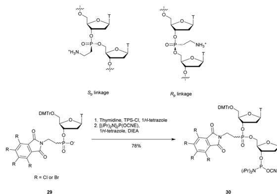
**Scheme 14** Chemical structures of *S<sub>p</sub>* and *R<sub>p</sub>* 2-AEP chiral linkages. Synthesis of the protected 2-(3,4,5,6-tetrabromophthalimido) or 2-(3,4,5,6-tetrachlorophthalimido) phosphoramidite building block **30**.
