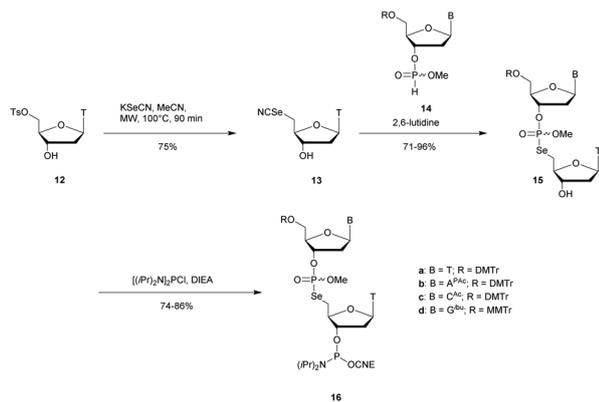
Scheme 10 Synthesis of phosphoroselenoate building blocks **16a-d**.<sup>151</sup>
