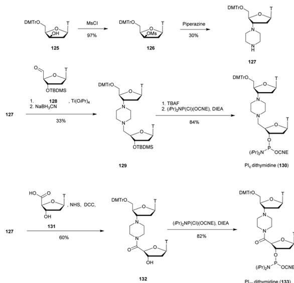
**Scheme 41** Synthesis of piperazine-dithymidine phosphoramidite building blocks **130** and **133** (PI<sub>c</sub> and PI<sub>co</sub>).
