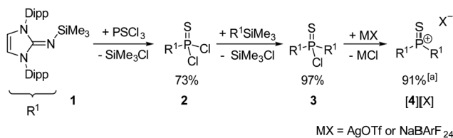
Scheme 2 Synthesis of [4][OTf] and [4][BARF 24 ] . Dipp = 2,6-diisopropylphenyl, OTf - = trifluoromethanesulfonate, BARF 24 - = tetrakis[3,5-bis(trifluoromethyl)phenyl]borate. a yield for MX = NaBARF 24 .
