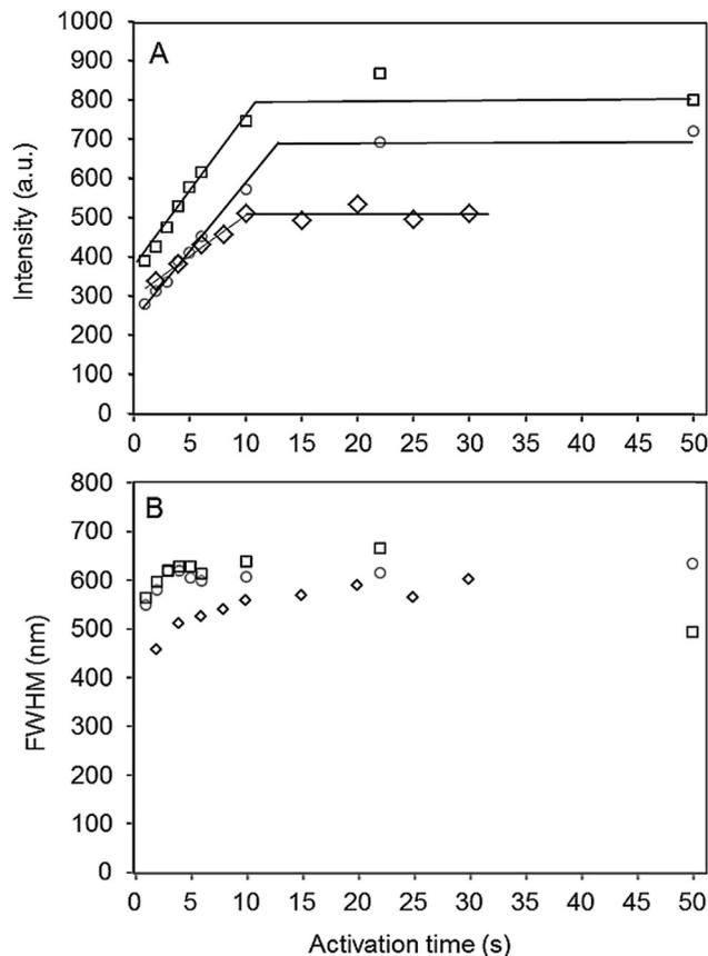
**Fig. 2** Intensity (A) and FWHM (B) of photo-activated carbon nanodots, given as a function of the activation time for 3 individual AlPO-5 crystals using  $9.5 \text{ MW cm}^{-2}$  as the activation power. The solid lines in Fig. 2A are only used to indicate the trends.
