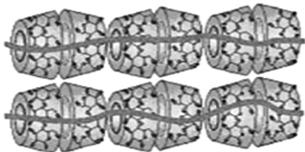
Scheme 11 Conceptual representation of the constrained polymerization of styrene molecules encapsulated within the narrow \gamma CD channels. The scheme has been reproduced from ref. 86 with permission from Wiley-VCH Verlag GmbH.
