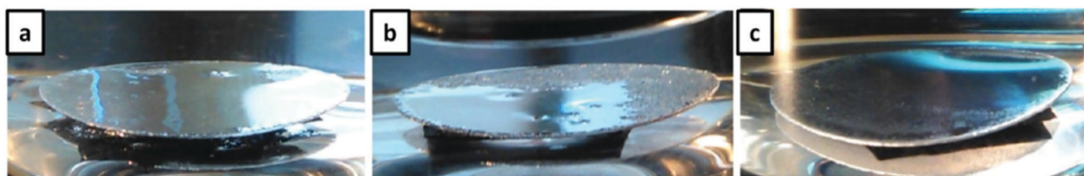
Fig. 40 Photos for coated substrates immersed in water for (a) a few minutes, (b) 100 hours, and (c) after removing and placing in the water again. (a–c) Reproduced with permission from ref. 187. Copyright (2017) American Chemical Society.
