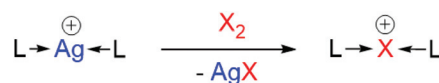
Scheme 1 A general method to synthesise halonium ions, facilitated by the strong driving force of the precipitation of AgX (spectator anions omitted for clarity).
