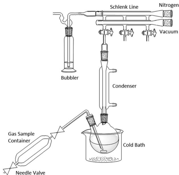
Fig. 12 Diagram of Grignard reaction apparatus. Note that the additional ports on the Schlenk line cannot be used during or immediately after this type of experiment.
