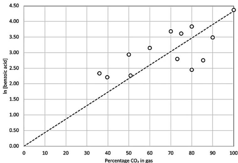
Fig. 9 Natural log of benzoic acid product concentration as a function of carbon dioxide concentration in the supply gas. Trend line projected back to point (0,0).
