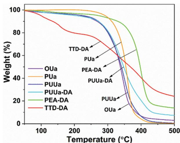
Fig. 4 The TGA curves of oligourea (OUa), polyurea (PUa), polyurethane-urea (PUUa), the polyurethane-urea Diels–Alder adduct (PUUa-DA), the poly(propylene glycol) bis(2-aminopropyl ether) Diels–Alder adduct (PEA-DA) and the 4,7,10-trioxo-1,13-tridecanediamine Diels–Alder adduct (TTD-DA).
