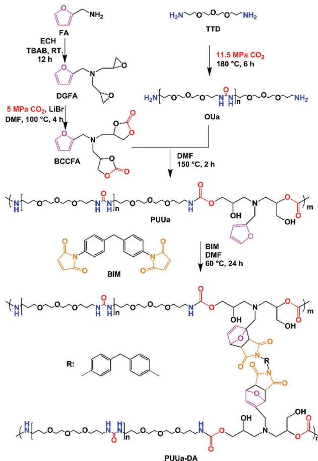
**Scheme 1** Synthesis of non-isocyanate polyurethane-urea (PUUa) from  $\text{CO}_2$ , and sequential transformation of PUUa with 4,4-bismaleimidodiphenylmethane to the polyurethane-urea Diels–Alder adduct (PUUa-DA).
