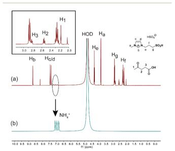
Fig. 8 <sup>1</sup>H NMR spectra (in D<sub>2</sub>O) of (a) reaction mixture of chitosan [C<sub>3</sub>SO<sub>3</sub>Hmim]HSO<sub>4</sub> catalysis and (b) standard NH<sub>4</sub>HSO<sub>4</sub>. Figure reproduced from ref. 61 with kind permission from Elsevier.
