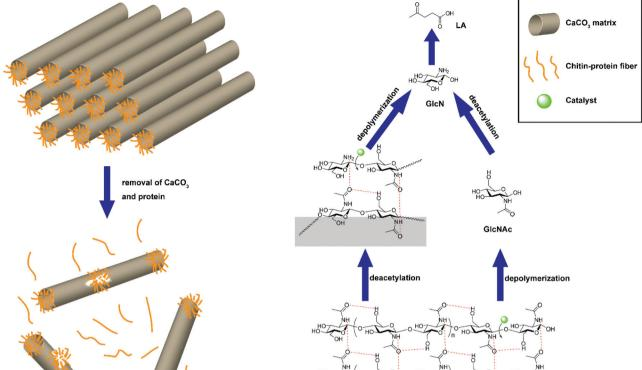
Fig. 5 Self-healing of chitin fraction during conversion of crab shells. Figure reproduced from ref. 64 with kind permission from the American Chemical Society.
