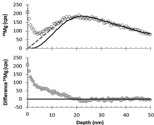
Fig. 8 Illustration of DLC surface correction using measured data (circles, SW\_3) vs. SRIM best fit (solid line) for the first 50 nm of the  $^{24}\text{Mg}$  depth profile. Top: comparison of raw data with the SRIM best-fit curve; dashed line gives an example of a (previously used<sup>10</sup>) visual correction based only on curve shape. Bottom: the difference between SRIM and the raw SIMS data.
