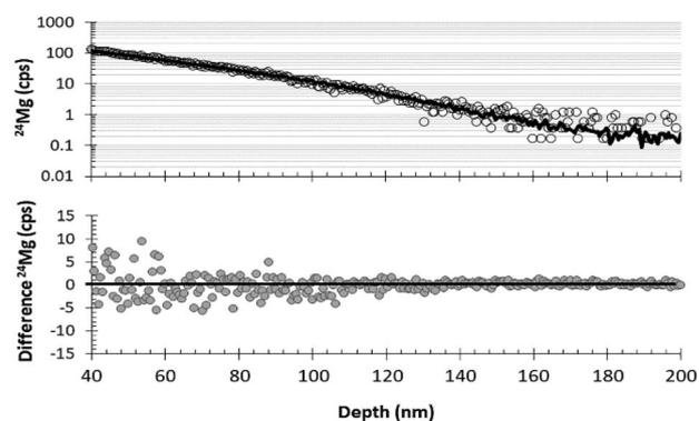
Fig. 7 Graphs demonstrating the quality of SRIM-fit to a measured DLC profile (SW\_3) for the last 160 nm of the  $^{24}\text{Mg}$  depth profile. Top: raw data (circles) plotted with SRIM best-fit curve (line); bottom: the difference between SRIM and the raw SIMS data.
