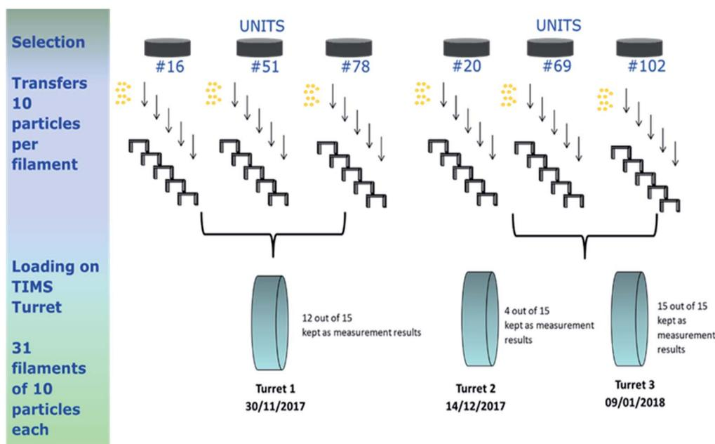
**Fig. 3** Flowchart of the analytical method used for the determination of the uranium amount per IRMM-2329P particle by ID-TIMS. Three TIMS turrets were prepared, since on turret 2, only 4 out of the 15 filaments could be retained for measurement results, due to inhomogeneity of the mixture between spike and sample in the other eleven filaments. In total, 31 measurement results were obtained/kept.
