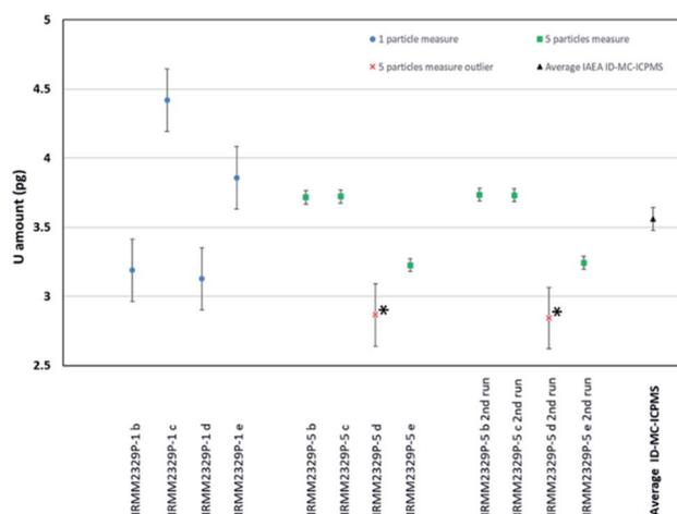
Fig. 9 Total U mass per particle and combined uncertainty ( $k = 1$ ) in IRMM-2329P reference material as measured at IAEA-SGAS using ID-MC-ICPMS. \*Note that the IRMM-2329P-5-d 1<sup>st</sup> and 2<sup>nd</sup> run samples were considered as containing only 1 particle instead of 5, and thus not taken into account into final average of the uranium amount.
