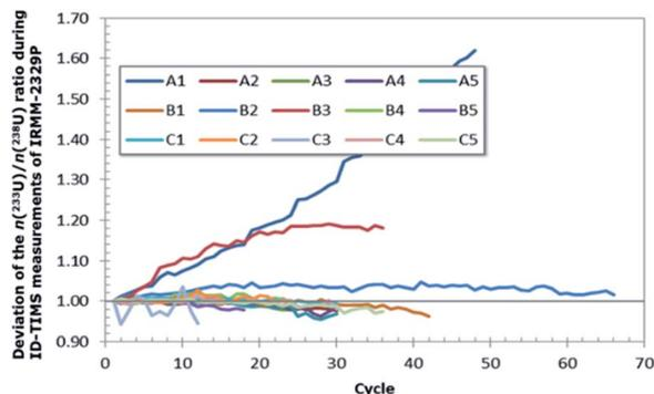
Fig. 5 TIMS measurements of the  $n(^{233}\text{U})/n(^{238}\text{U})$  ratio of filaments of the first IRMM-2329P turret, showing the drift of the measured  $n(^{233}\text{U})/n(^{238}\text{U})$  ratio from the initial  $n(^{233}\text{U})/n(^{238}\text{U})$  measured at the beginning of the measurement cycle. It can be seen on the graph that only two filaments (A1 and B3) showed a drift exceeding 10% of the initial value, and were therefore discarded as outliers.
