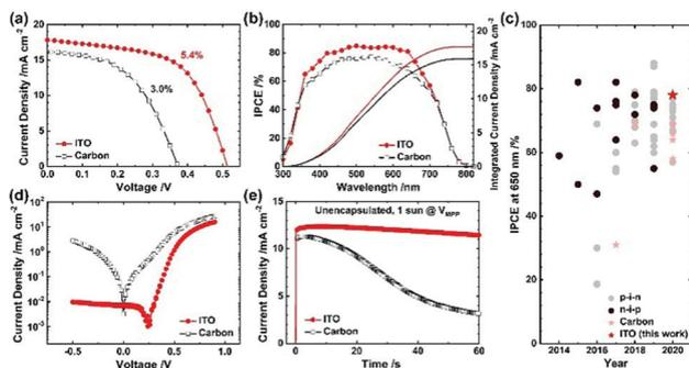
Fig. 4 Comparison of ITO and carbon devices. (a)  $J$ - $V$  curves measured under standard one-sun conditions. (b) IPCE spectra. (c) Evolution of IPCE (at 650 nm) of the inverted (p-i-n), regular (n-i-p), carbon and ITO devices. (d)  $J$ - $V$  curves measured under darkness. (e) Output current density measured under the standard one-sun conditions, at maximum power point and under ambient air.
