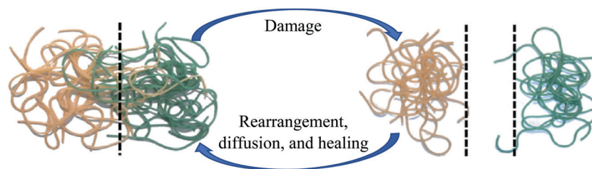
Fig. 13 Schematic of physical self-healing process [reproduced from ref. 136 with permission from the Wiley].
