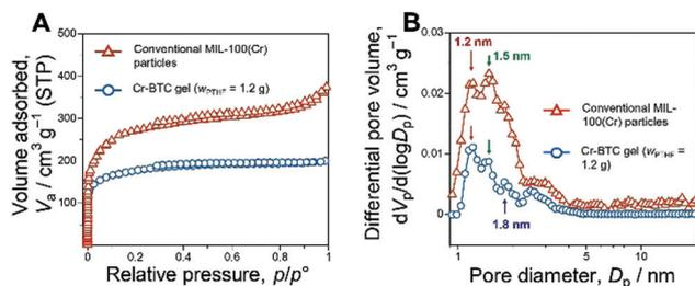
**Fig. 3** Micro-/mesoporous structures of the as-dried macroporous Cr-BTC gel and the conventional MIL-100(Cr) particles. (A) Nitrogen adsorption–desorption isotherms of the samples and (B) pore size distributions obtained by NLDFT analysis. The BET surface area of conventional MIL-100(Cr) particles is calculated to be  $1050 \text{ m}^2 \text{ g}^{-1}$ .
