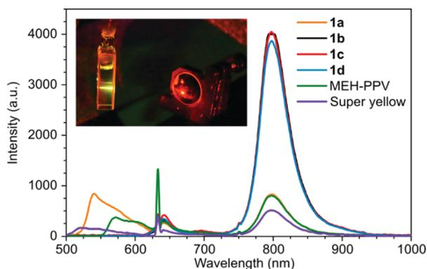
Fig. 3 Emission spectrum of samples containing copolymers **1a–d** (0.25 mg mL<sup>-1</sup>), MEH-PPV (0.5 mg mL<sup>-1</sup>), super yellow PPV (0.5 mg mL<sup>-1</sup>) with PdTPTBP (7.5  $\mu$ M) as the sensitizer in chloroform solution under 632 nm excitation. Phosphorescence of PdTPTBP was observed at 800 nm and the upconverted emission was observed at 500–600 nm. The insert is a photo of a cuvette containing copolymer **1a** and PdTPTBP showing yellow TTA-UC emission.
