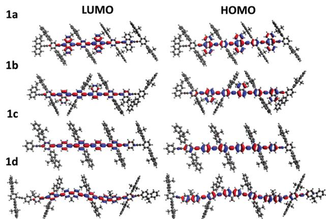
Fig. 5 DFT calculations of model oligomers of **1a–d** displaying the electron probability distributions for the highest occupied molecular orbitals (HOMO) and lowest unoccupied molecular orbitals (LUMO) for various aryl comonomer units.
