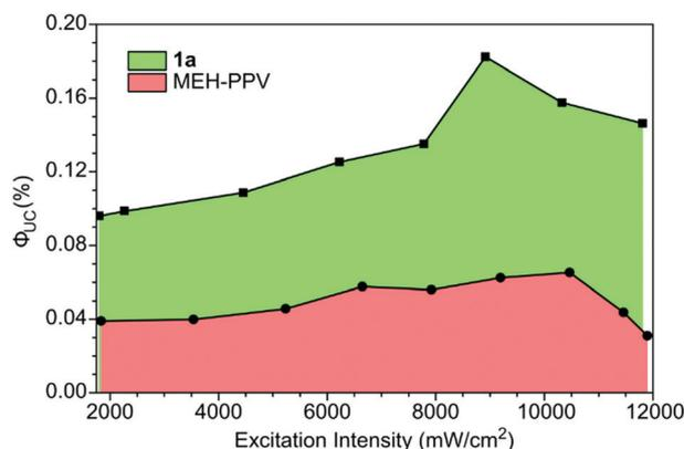
Fig. 4 Dependence of upconversion quantum yield on excitation intensity for PPE **1a** (0.25 mg mL<sup>-1</sup>), MEH-PPV (0.5 mg mL<sup>-1</sup>) with PdTPTBP (7.5  $\mu$ M) as the sensitizer in chloroform solution under 632 nm excitation.
