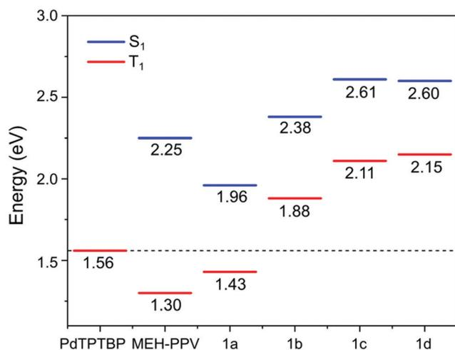
Fig. 6 Energy diagram depicting the calculated singlet and triplet excited state energies obtained by DFT of the model oligomers of **1a–d** compared to the triplet excited state energy of PdTPTBP. The values for MEH-PPV are taken from ref. 34.
