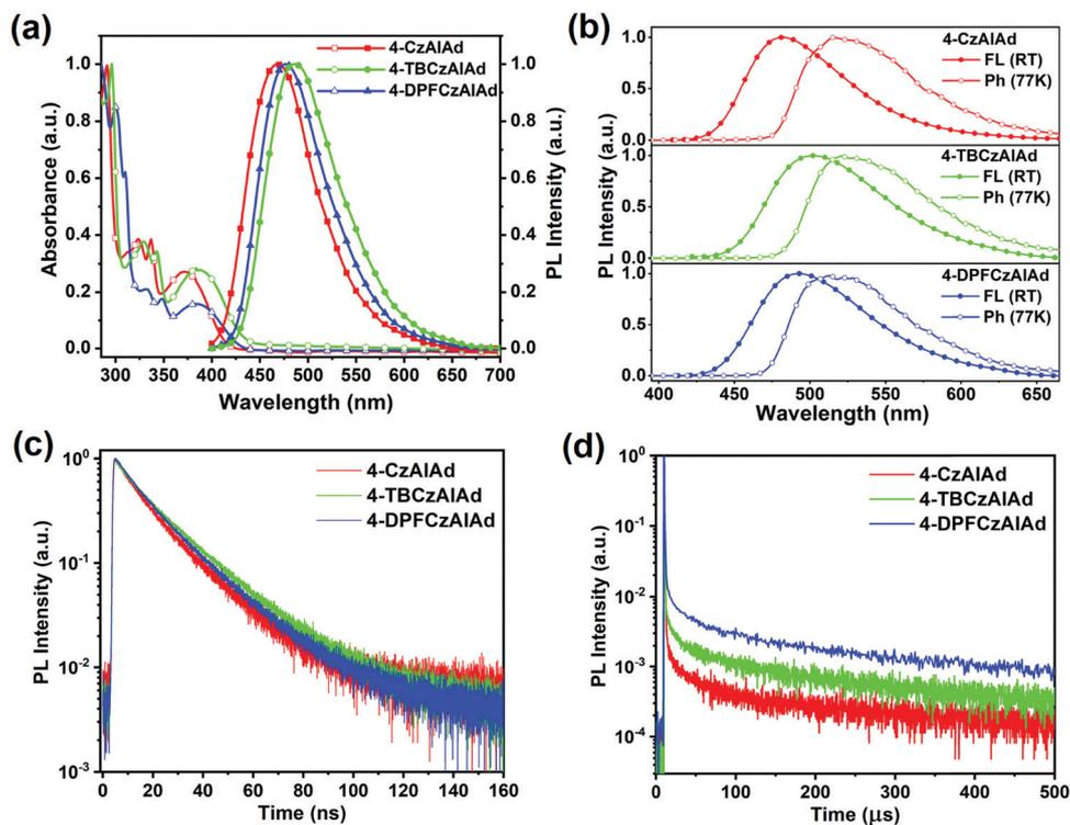
Fig. 3 (a) UV-vis absorption and PL spectra of the three emitters in toluene solution ( $10^{-5}$  M). (b) PL spectra and phosphorescence spectra of the three emitters in doped films. (c) The prompt decay curves and (d) delayed decay curves of the three emitters in doped films.
