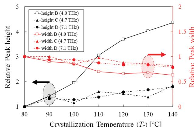
Fig. 3 Relative height and width of peaks B, C, and D plotted against the crystallization temperature, normalized at 80 °C. Absolute height (width) of peak B, C, and D at 80 °C are  $4.78 \text{ cm}^{-1}$  (0.36 THz),  $9.38 \text{ cm}^{-1}$  (0.56 THz), and  $25.13 \text{ cm}^{-1}$  (0.46 THz), respectively.
