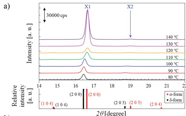
Fig. 4 (a) XRD profiles of PLLA for different crystallization temperature, and standard XRD data of polylactide (JCPDS card no. 64-1623 for  $\delta$ -form and 64-1624 for  $\alpha$ -form). (b) Diffraction angle  $2\theta$  of the two peaks labeled in (a). The lattice spacing  $d_{hkl}$  values with the Miller indices, calculated by the Bragg equation, are superimposed.
