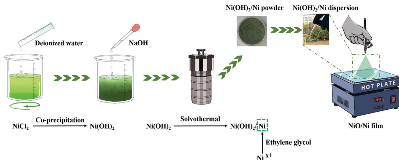
Fig. 1 Schematic illustration of the preparation of the NiO/Ni electrode.
