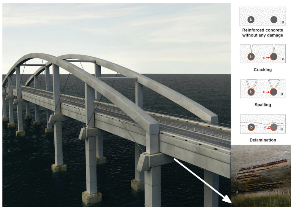
Fig. 3 Bridge with a schematic representation of cracking, spalling or delamination in a RCS where “a” represents the concrete, “b” the rebar and “c” the oxide layer. The photograph in the bottom right corner shows the typical feature of concrete detachment due to rebar corrosion.
