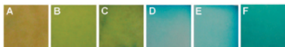
Fig. 31 Visual color changes of probe-97-coated paper strips with different amounts of PA; the [PA] values are (A) 10^{-2} M, (B) 10^{-4} M, (C) 10^{-6} M, (D) 10^{-9} M, (E) 10^{-11} M, and (F) no PA. Reprinted from ref. 101, Copyright 2013 Royal Society of Chemistry.
