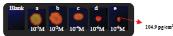
Fig. 28 Probe- 84 -coated paper strips upon interaction with different concentrations of PA [(a) 1.049 mg, (b) 0.1049 mg, (c) 1.049 \mu\text{g} , (d) 10.49 ng, and (e) 104.9 pg]. Reprinted from ref. 92, Copyright 2015 Royal Society of Chemistry.
